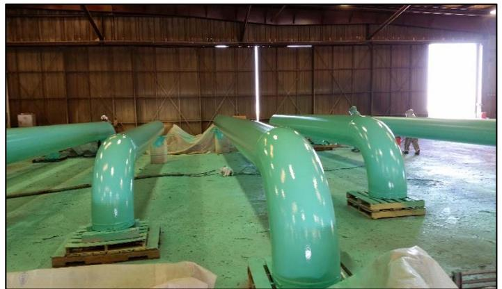
The fabricated specials drastically reduced the amount of field work required. Enviroline® 376-60 was used for road crossings due to its abrasion resistant abilities.
