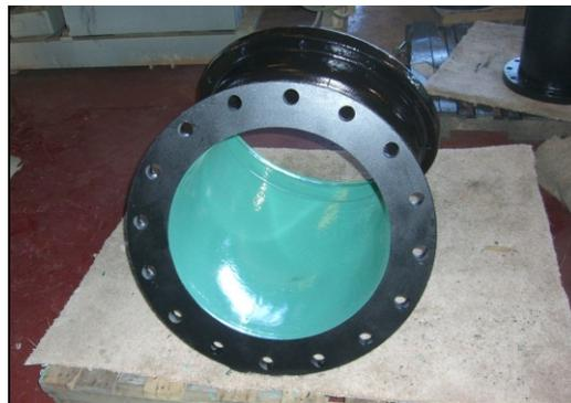
Fusible PVC™ pipe with coated and lined ductile iron fittings at the project site
