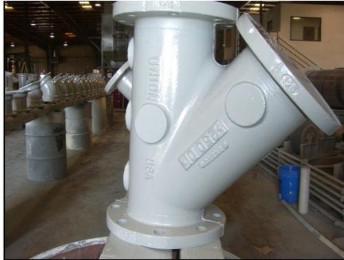
Finished fittings lined with Tnemec® 431 (green) and Americoat® 385/78HB coal tar epoxy coating
