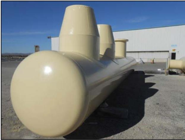
**Figure 1: Finished 54" Header Assembly.** This special project consisted of over 225 special spool pieces that were coated with the epoxy and polyurethane.
