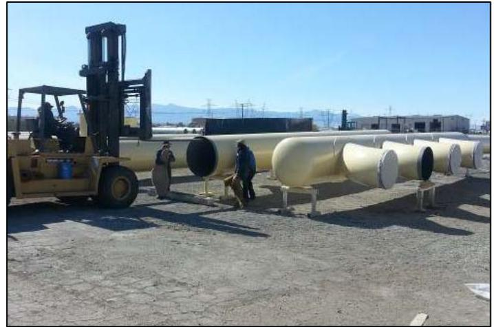
**Figure 2: Mobile Pipe performed quality assurance testing and capped the ends.**
