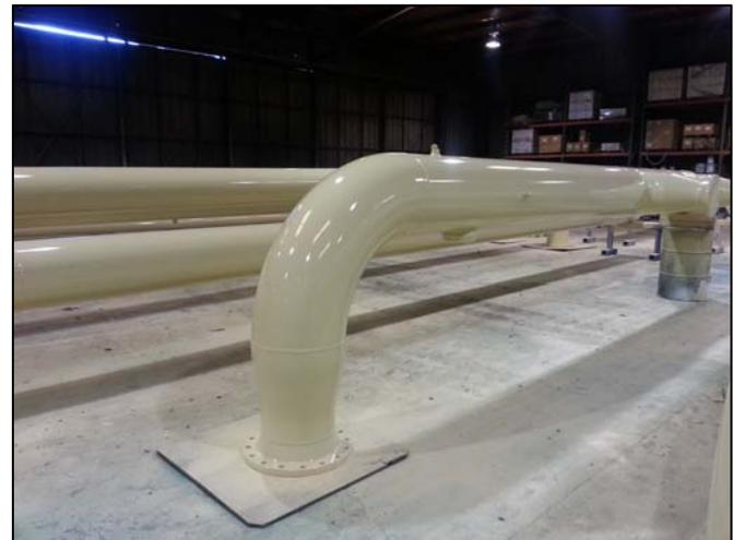
**Figure 4: Fabricated specials coated and set aside to cure.** Mobile Pipe has an enclosed 36,000 ft<sup>2</sup> facility to control environmental factors and eliminate rework – resulting in on-time deliveries.
