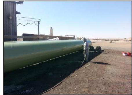
Polyclad 975 is a 100% solids epoxy applied at 20 mils nominal thickness. It is designed as an alternative to FBE. [For more information click here](#)
