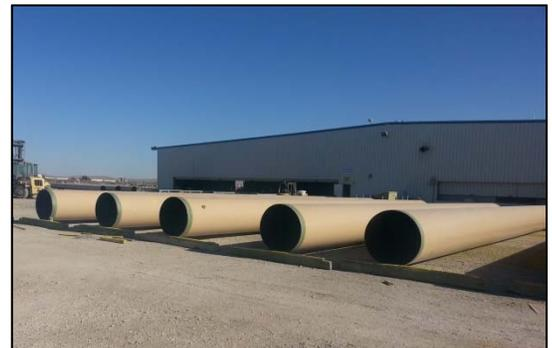
Utilizing automated production schedules, Mobile Pipe was able to process the order in under three weeks. The pipe leaves the facility 100% holiday free.
