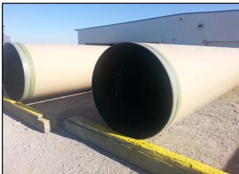
The 42" casing pipe also received 3 mils of Carbothane® 134HG for UV protection. Both the 975 and 134HG product can be applied in the field for joint protection.
