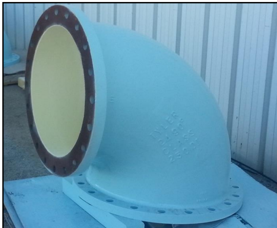
24" Ductile Iron 90° fitting lined with 40 mils of LifeLast Durashield™ 210 and coated with Sherwin Williams zinc/epoxy/urethane system for UV exposure.
