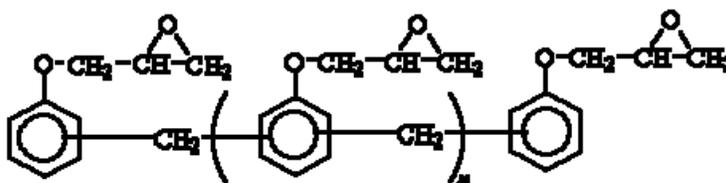
Figure 1: Chemical Structure of Novolac Epoxy Resin
