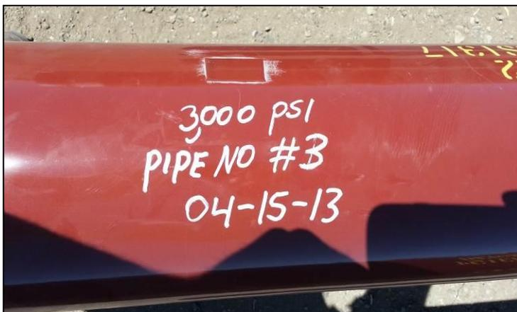
Each pipe is tested via ASTM D4541 for proper adhesion. This test shows a value of 3,000 PSI. Once the dolly is removed, the coating is sanded then patched.
