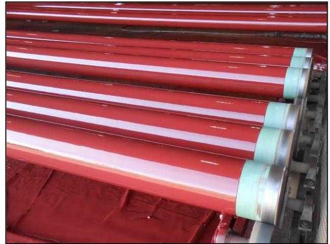
Powercrete® R-60 applied at 35mils. The pipe is positioned on rotating wheels and Powercrete® is spray applied. The coating is then checked with a wet film thickness gauge (WTF) and allowed to cure. Once cured, it is checked with a dry film thickness (DFT) gauge to verify specification compliance. Once the hardness reaches 78 Shore D, the pipe is ready to be handled and tested for holidays and proper adhesion.
