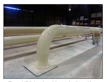
Figure 4: Fabricated specials coated and set aside to cure. Mobile Pipe has an enclosed 36,000 ft<sup>2</sup> facility to control environmental factors and eliminate rework – resulting in on-time deliveries.
