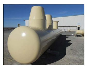
Figure 1: Finished 54" Header Assembly. This special project consisted of over 225 special spool pieces that were coated with the epoxy and polyurethane.
