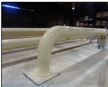
Engineers learn how fabricated specials can save time and cost as well as pipe sizes that can be lined and coated and then shipped to the job site
