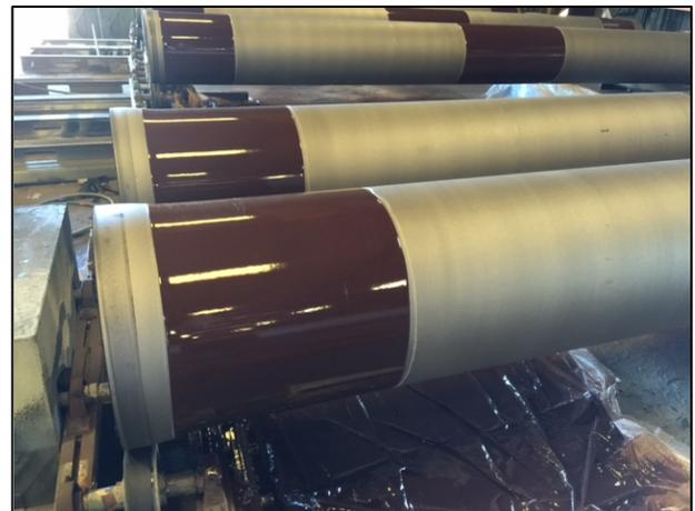
Powercrete® J is applied per AWWA C210 with a minimum thickness of 20 mils. The steel is blasted per SSPC SP-5. This process occurs after the pipe is cement mortar lined per AWWA C205.
