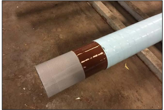
Since the AWWA C225 polyethylene was melted and cooled in Mobile Pipe's factory controlled environment, there is no risk of shrink-back.
