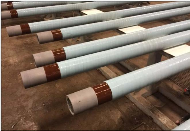
A 6-inch holdback is left for field connection, while the AWWA C225-compliant SYNERGY® coating system is applied over the top of the 18-inch Powercrete® J extending the entire length of the pipe.
