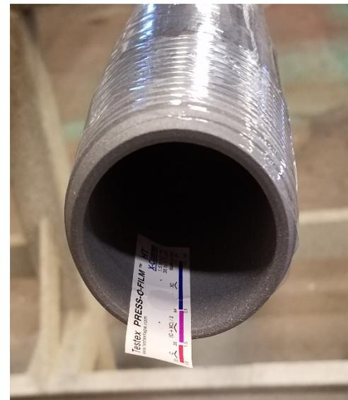
**Figure 2:** While not the only critical quality parameter, achieving a blast profile of 2.5-3.5 mils is essential in preparing the surface for proper adhesion of the epoxy.
