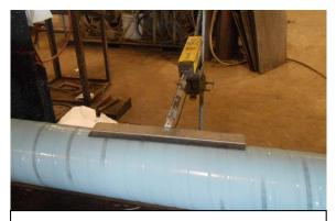
Factory automated holiday detection ensures that the coating is properly adhered to the pipe substrate and helps eliminate voids.
