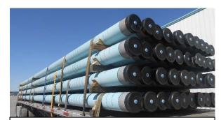
Ensuring the product is applied holiday-free is only the first step. Proper loading, including capping, padding and equal weight distribution between dunnage is key to reducing shipping damage.
