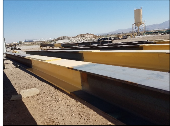
Figure 4: Mobile Pipe's 40-acre facility is more than adequate to handle the 60-foot H-piles. Our modern equipment enables Mobile Pipe to apply the polyurethane in a consistent and reliable manner.
