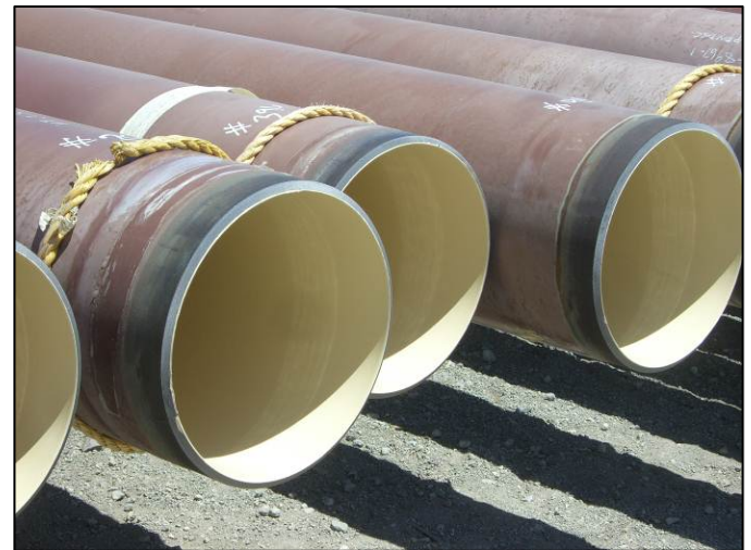
Pipe ready for holiday testing per NACE SPO188-06. In total, 627 joints were tested. Mobile also repaired coating damage to the dual layer FBE to protect the abrasion resistant overlay.
