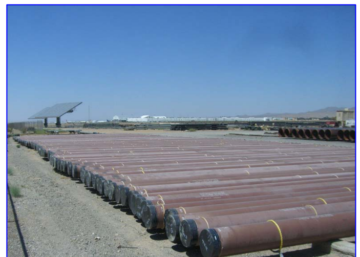
Mobile Pipe stripped and relined over 28,000 LF of steel pipe.
