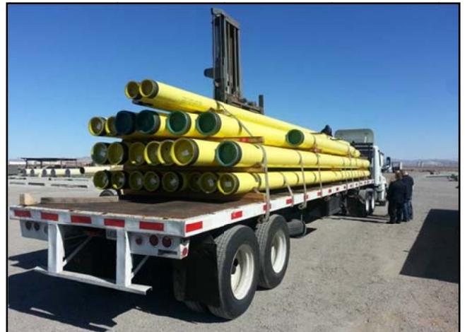
Portions of the Synergy® coated pipe loaded with end caps for protection. In addition to natural gas transmission, Synergy® can be used for water distribution and transmission lines
