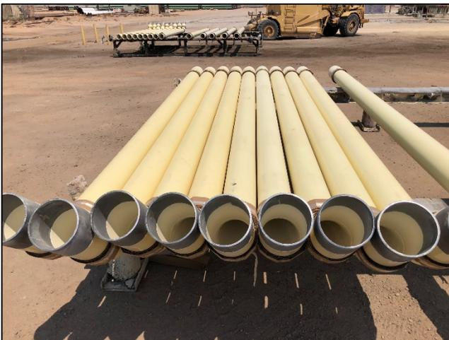
Mobile Pipe can accommodate pipe up to a 40-foot in length, with one bend on the end, having an inner diameter as small as 4 inches and an unlimited outer diameter. Prefabricated specials lined and coated by Mobile Pipe for the Cobbs Creek Reservoir are pictured.
