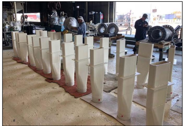
DuraShield™ 210-61 polyurethane is available in two cure speeds that produce a tack-free surface within 15 to 45 minutes following application. The cure speed of polyurethanes significantly decreases production time associated with painting fabricated pieces.
